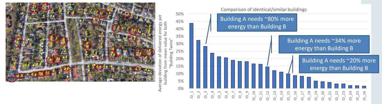
In 12 out of 26 "twin building" cases (2x26 buildings) in this area, the delivered energy of one building exceeds that of the second by more than 1/3 (with a median value of 25%).
