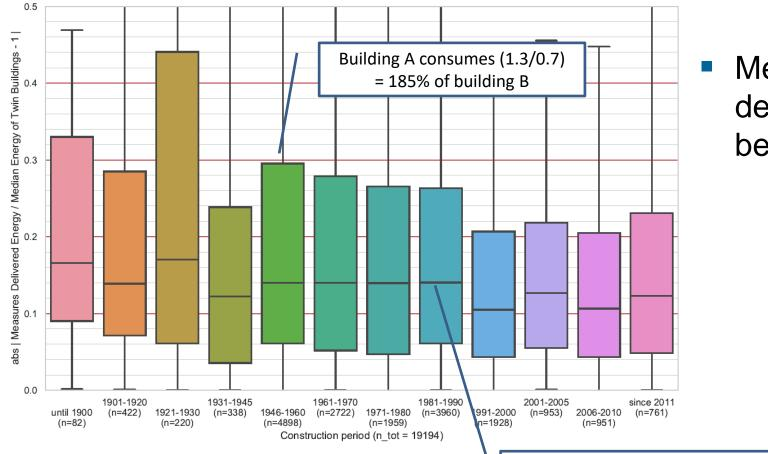
Median level for deviation in delivered energy between twin buildings is ~33%.
