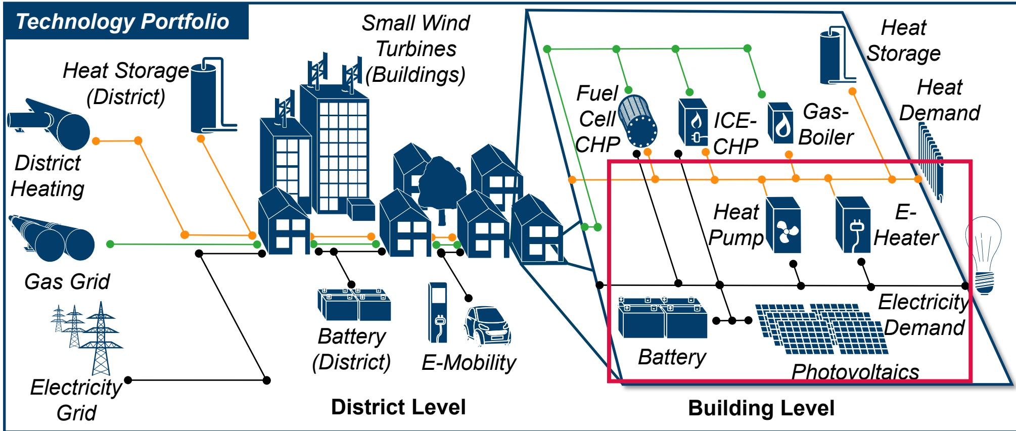
**Design and operation optimization** for cost optimal district energy supply system under consideration of various **sector-coupling options** and an increasing **integration of electric mobility**
