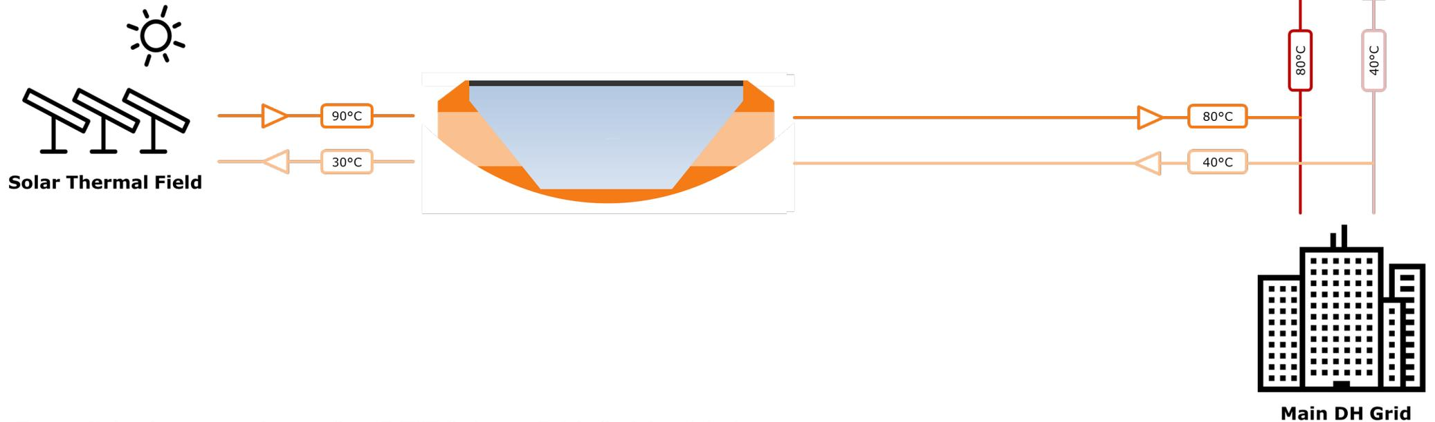
*Possible Integration of a PTES in a DH Grid with low temperatures*
