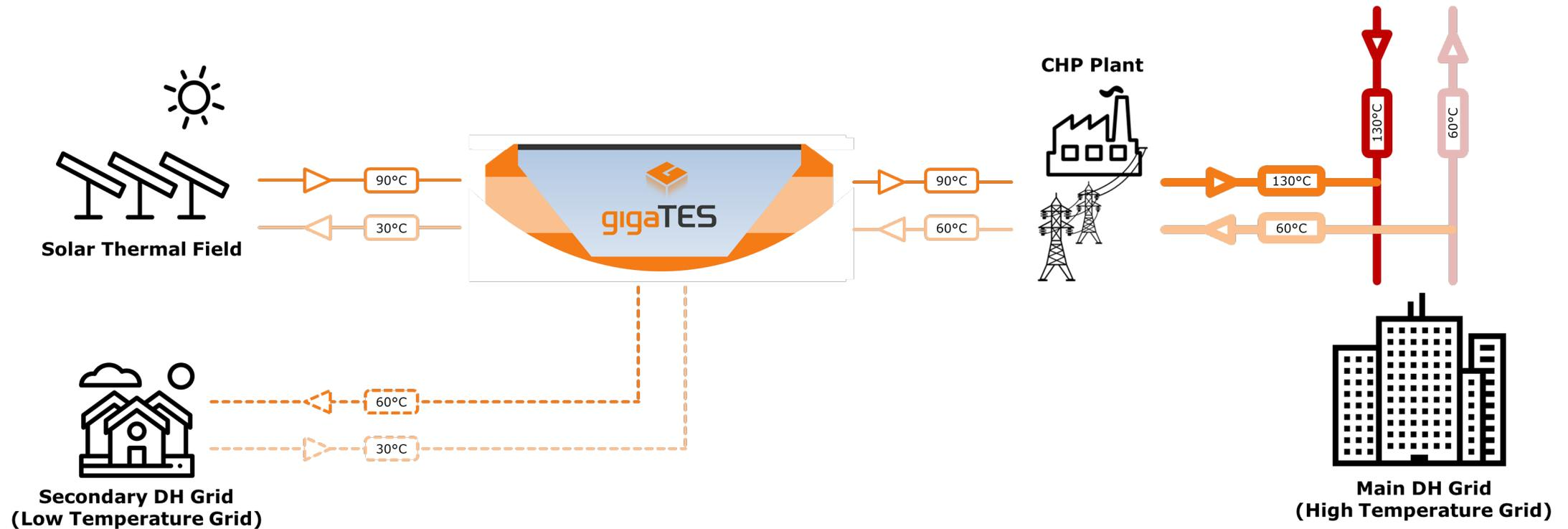
*Possible Integration of a giga\_TES in a DH grid with high temperatures*
