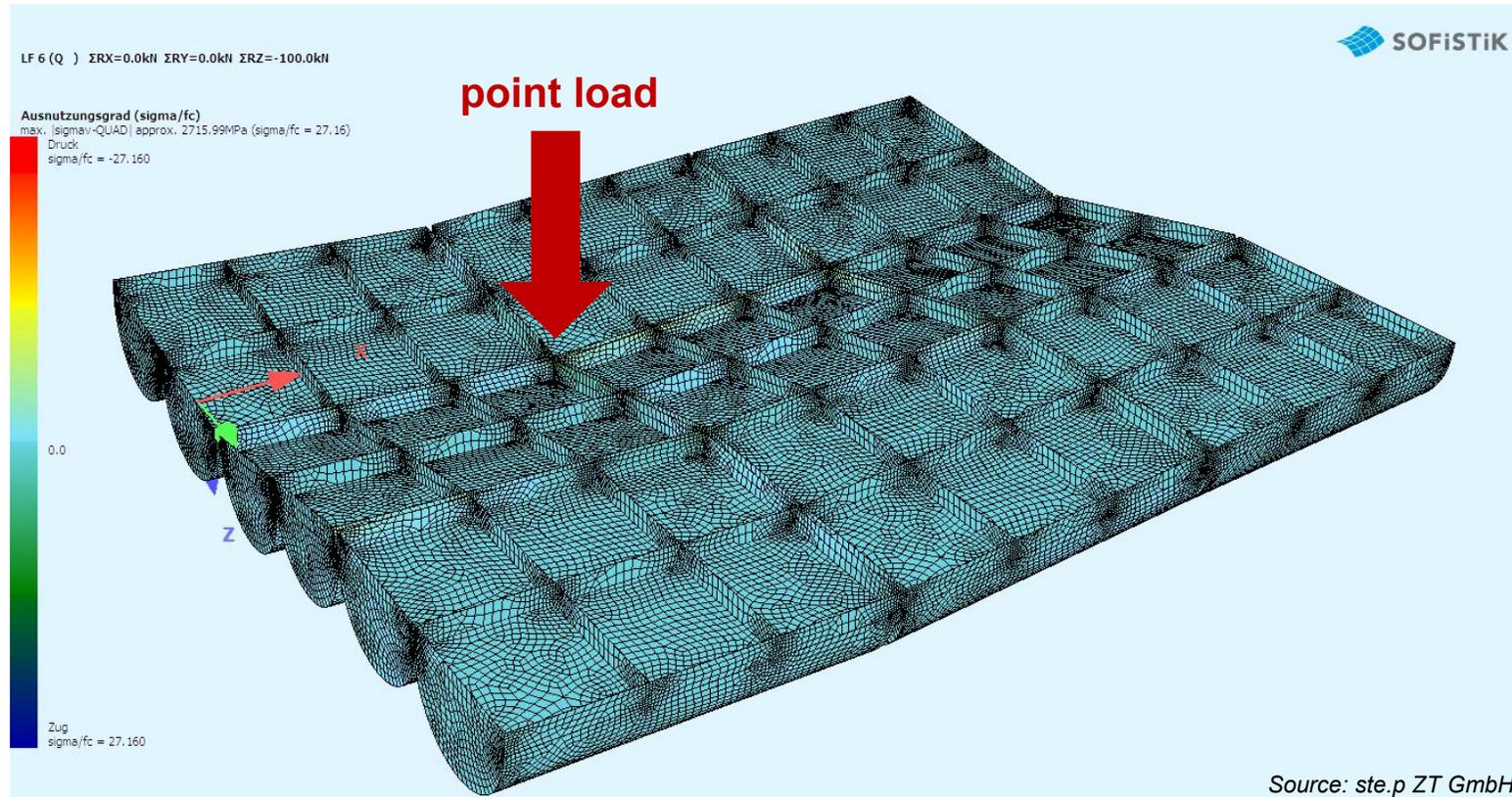
*FEM analyses of a possible cover construction with floating pontoons stressed with a point load*
