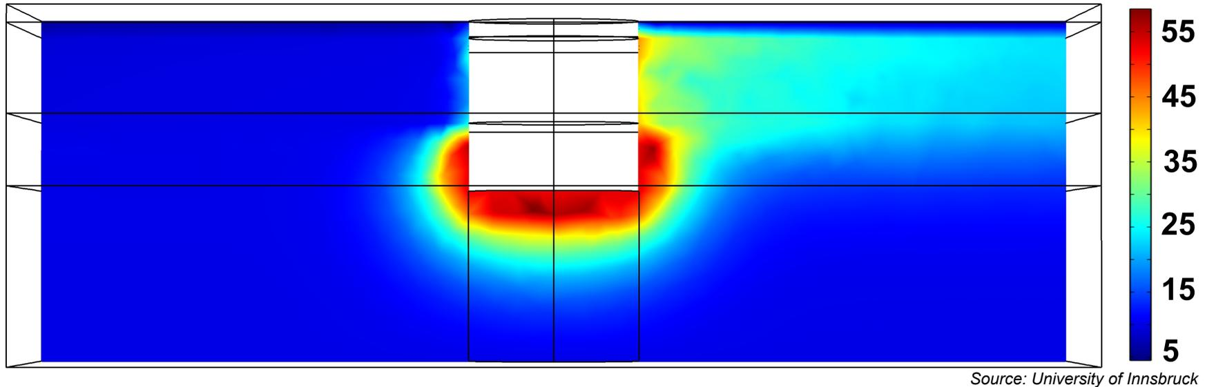
*2D simulated temperature field (in °C) of the surrounding subsurface of a storage with groundwater flow*
