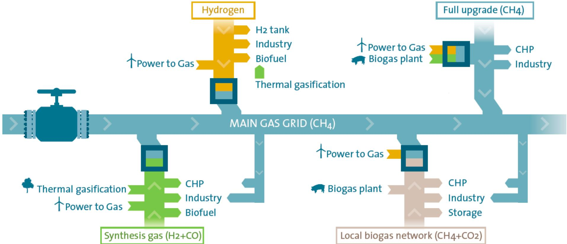
New types of RE gasses to be integrated – essential to handle sub-nets with other gas-specification
