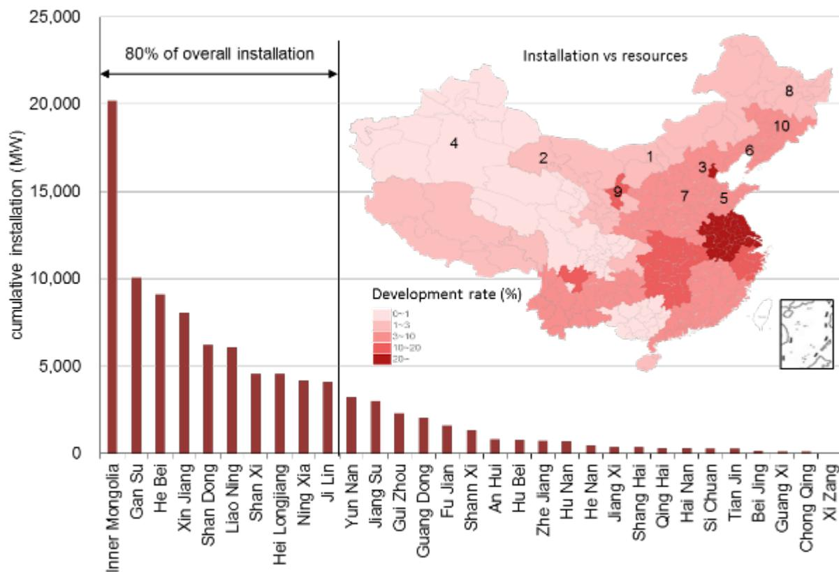
The Northeast Grid region accounted more than 30% of China's total wind capacity, but contributed almost 50% of total wind power curtailment.
