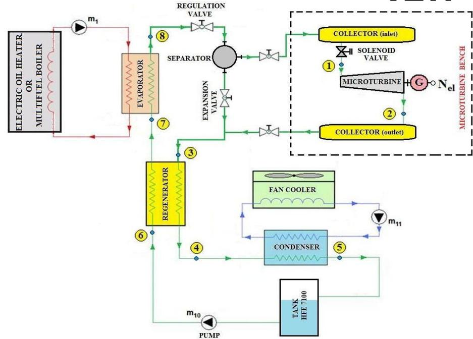
**Fig. 2.** Diagram of the ORC installation equipped with a radial microturbine [1]
