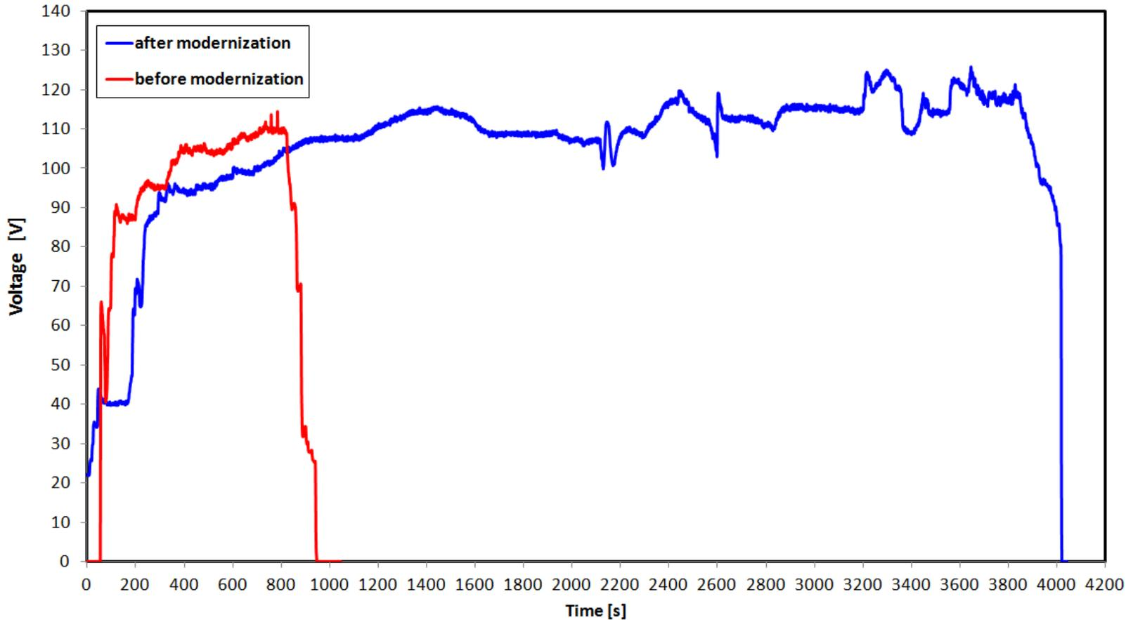
**Fig. 8.** Voltage generated by the microturbine (before and after its modernization) vs. time
