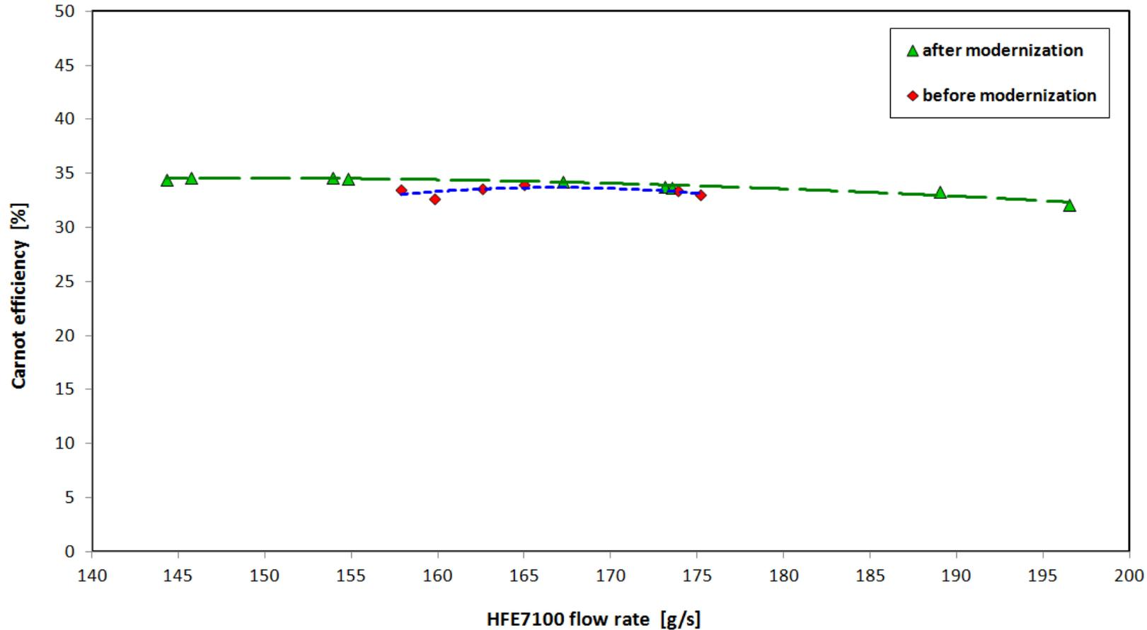
**Fig. 17.** Carnot efficiency vs. HFE7100 flow rate
