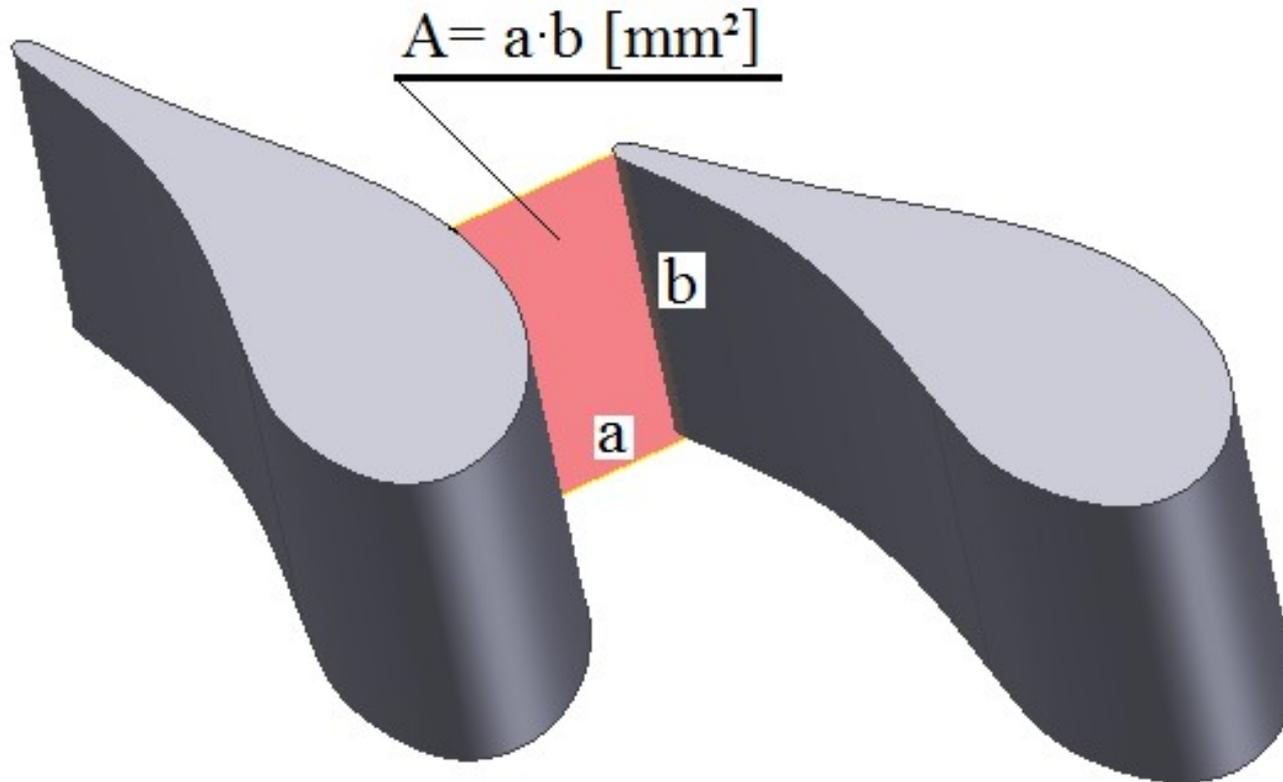
**Fig. 5.** Geometry of the microturbine wheel vanes and the cross sectional area of the delivery channel
