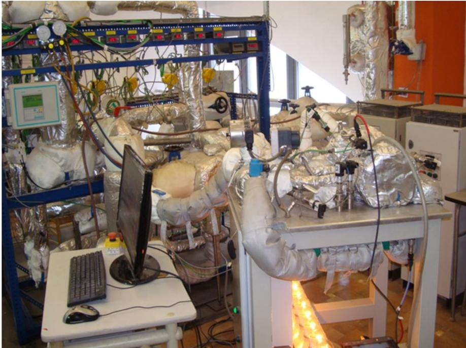
**Fig. 1.** Photo of the ORC installation operating with a radial microturbine [1]
