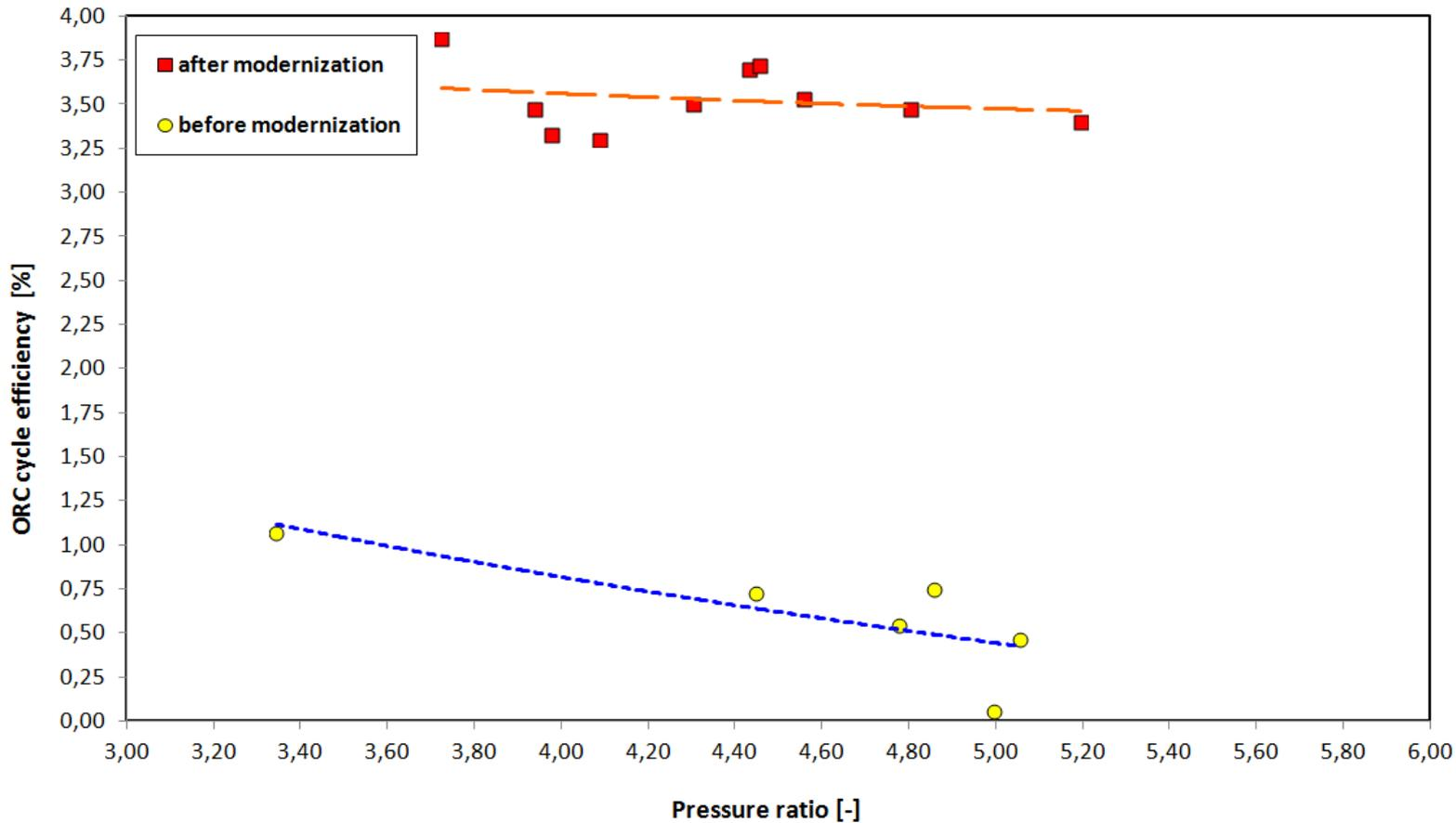
**Fig. 15.** ORC cycle efficiency vs. pressure ratio
