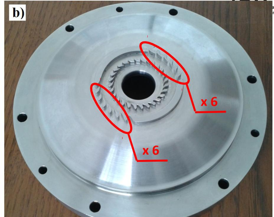
Fig. 4. Photo of the microturbine wheel: a) before and b) after the modernization
