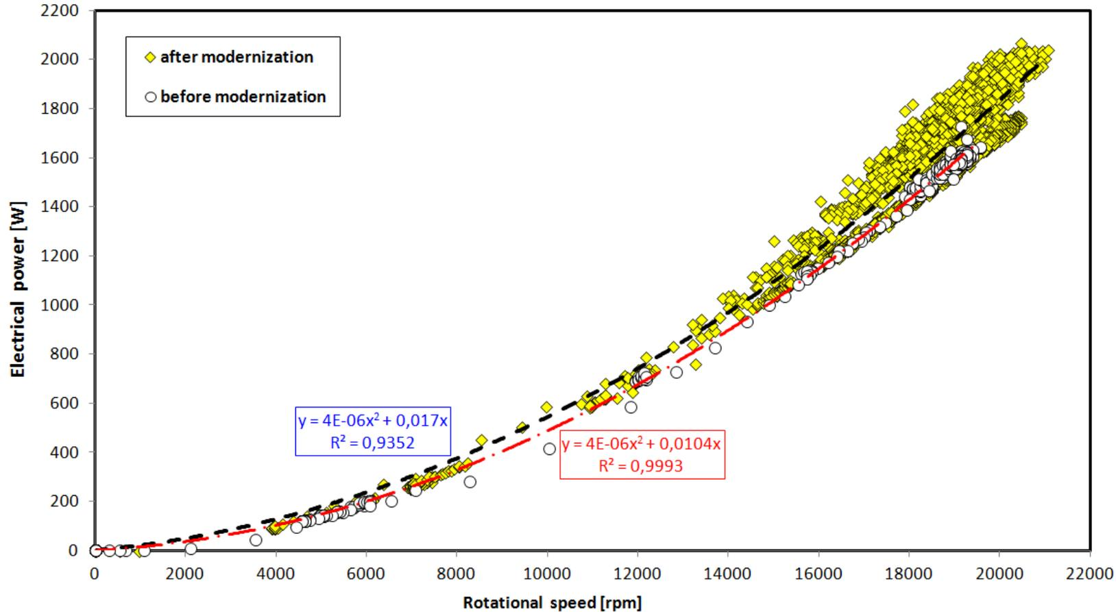
**Fig. 7.** Electrical power generated by the microturbine (before and after its modernization) vs. rotational speed
