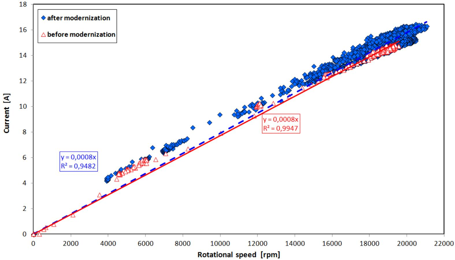
Fig. 11. Load current of the microturbine (before and after its modernization) vs. rotational speed
