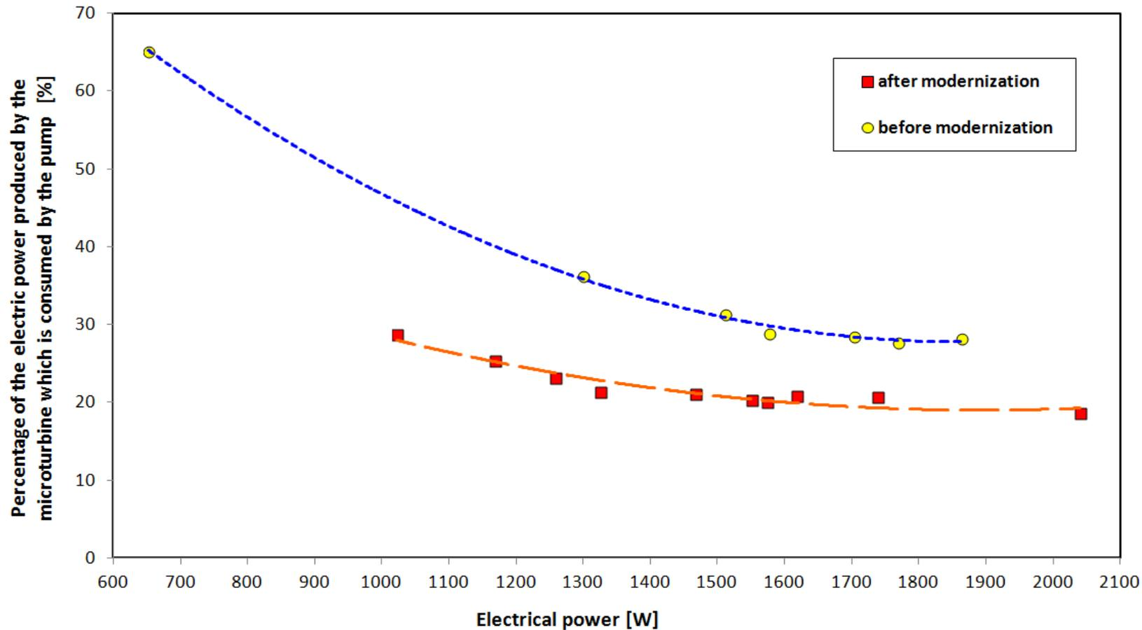
**Fig. 20.** Percentage of the electric power produced by the radial microturbine which is consumed by the pump vs. electrical power (before and after the microturbine modernization)
