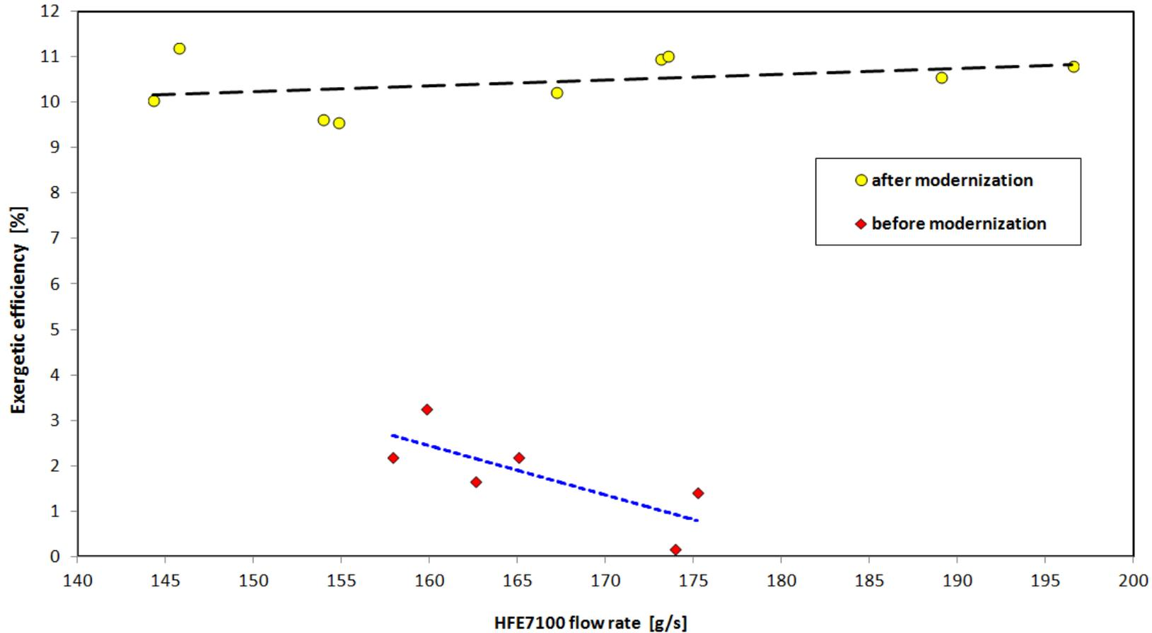
**Fig. 19.** Exergetic efficiency vs. HFE7100 flow rate
