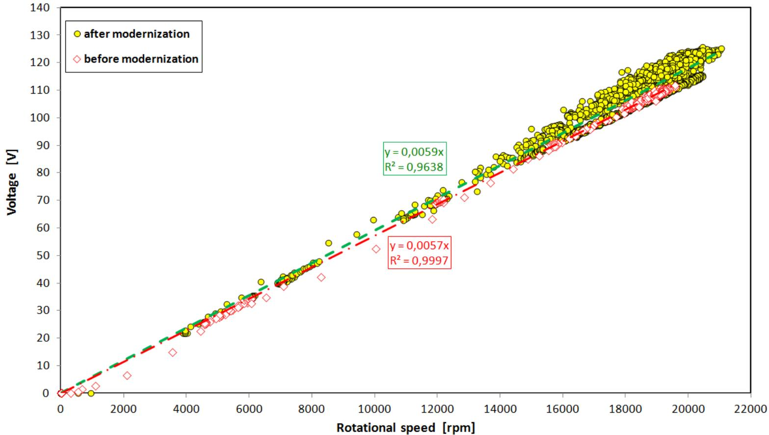
Fig. 10. Voltage generated by the microturbine (before and after its modernization) vs. rotational speed
