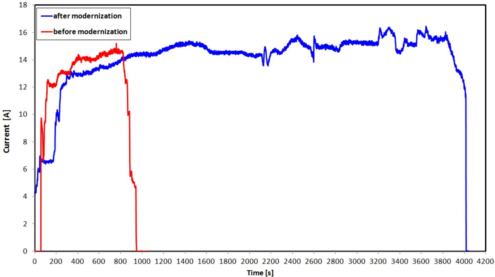
**Fig. 9.** Load current of the microturbine (before and after its modernization) vs. time
