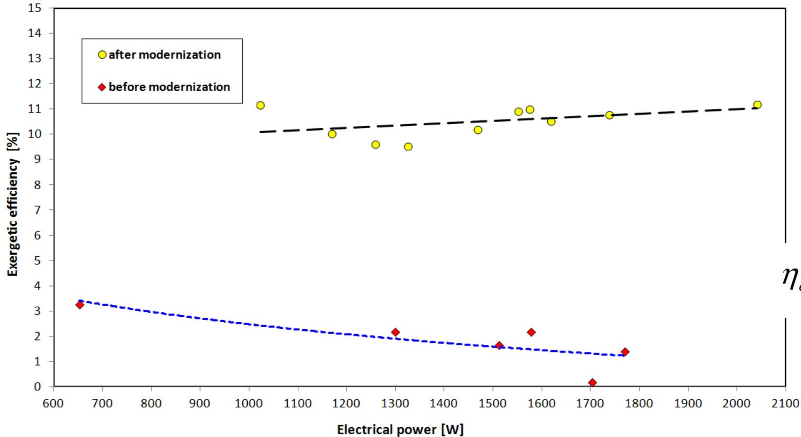
**Fig. 18.** Exergetic efficiency vs. electrical power generated by the microturbine (before and after its modernization)
